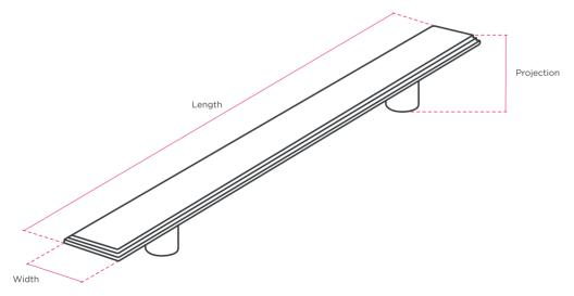
Fixings: Supplied 2x M4 x 30mm machine bolts
