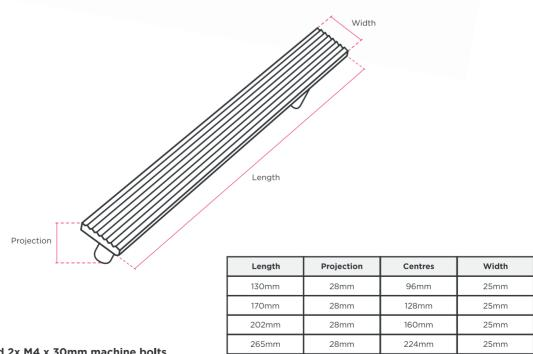
Fixings: Supplied 2x M4 x 30mm machine bolts
