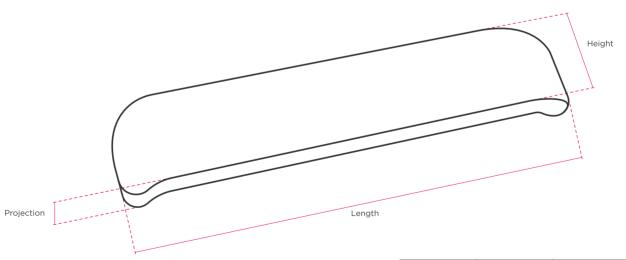
Fixings: Supplied 2x M4 x 30mm machine bolts
