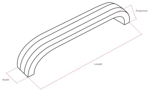
Fixings: Supplied 2x M4 x 30mm machine bolts
