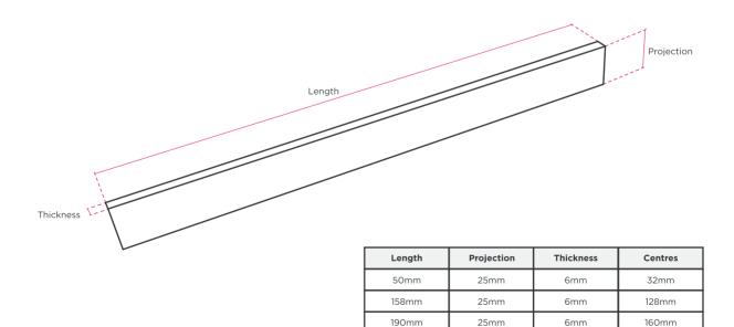
Fixings: Supplied 2x M4 x 30mm machine bolts
