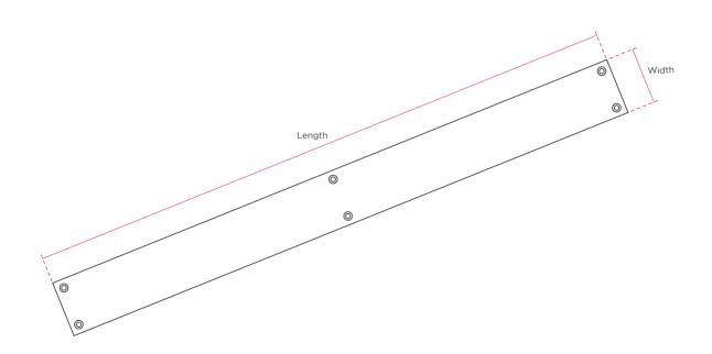
Fixings: 6 x Semi domed slotted screws no.6 x 1"
