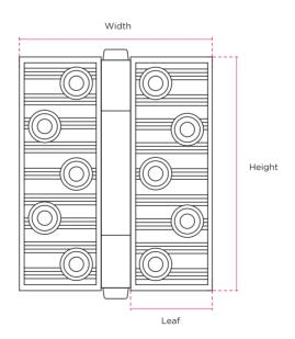
Sold Individually with matching screws. Max. Load Bearing 160kg based on 3 hinges per door.
